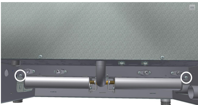
Unscrew the screws of the left and right burner.
