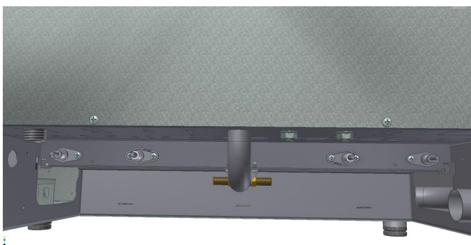
After removing the burners, burner nozzles unscrew the two left and two right of burner nozzles.
