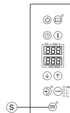
If the door is opened during preheating (before reaching the set preheating temperature), preheating is automatically interrupted, as it is presumed the food has been loaded into the oven.
